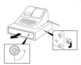
The drawer will automatically open on appropriate operations. However, in the event of a power failure, etc., the drawer can be released manually.
